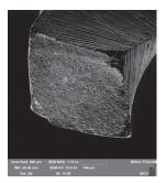
Fig 5. Size 20.06 and 20.07 files after cyclic failure
