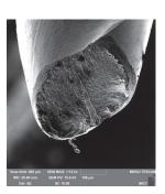
Fig 4. Size 15.03 and 20.04 files after cyclic failure
